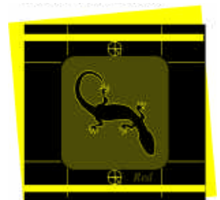
Figure 2: By viewing negatives one by one (left and center), it is difficult to gauge trap. Viewing both negatives with a transparent yellow overlay between them (right) allows for a simple, accurate method of checking of trap.
